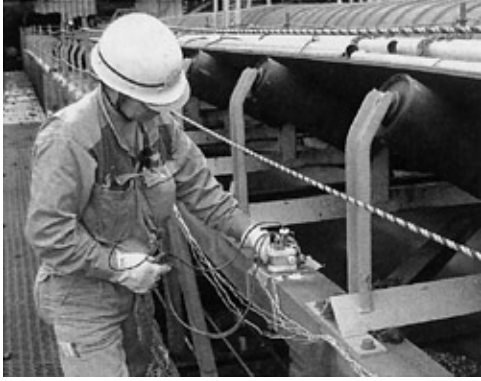
Photo 2 Stress measurement using the system
